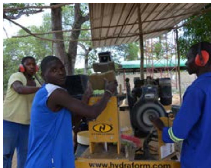
Figure 5B.2 YA Dondo - brickmaking machine
