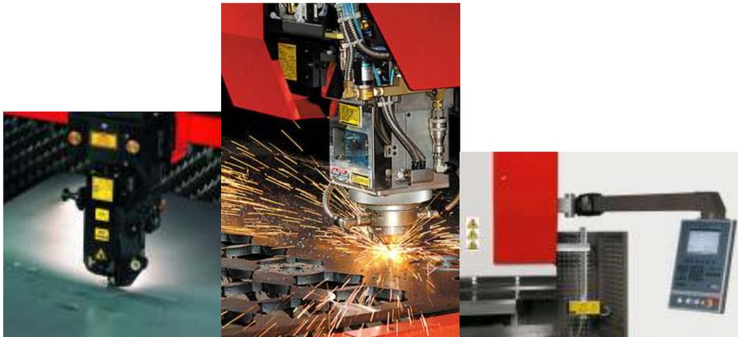
This ensures the combined approach of punching of metal components with the flexibility and quality of laser cutting in one combined manufacturing operation. Components are therefore consistently accurate within close tolerances.
